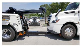
11. Secure the vehicle axle to the tow truck crossbar with a chain or ratchet strap.
