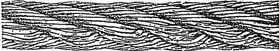
This is an illustration of a serious condition where the rope slides over or against itself.
