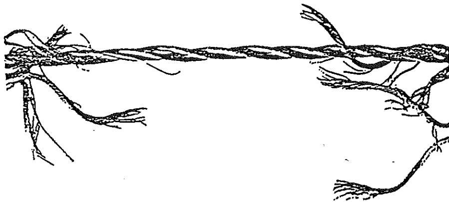
This is the appearance of a typical lension break: a result of overloading.
